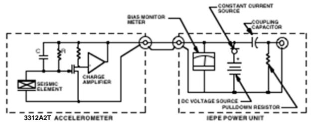
**Figure 1 - Electro-mechanical schematic, accelerometer and power unit system.**
