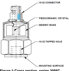
The seismic masses, made from a very dense tungsten alloy, and are tightly preloaded against the ceramic crystals by means of a special preload screw, to a flat crystal support, under hundreds of pounds of force. This is so there is absolutely no relative motion between mass, crystals and base keeping the nonlinearity low and the natural frequency high.
