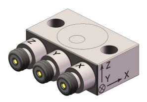
Model 3443C is a charge mode triaxial accelerometer featuring 3 separate 10-32 connectors mounted in a titanium housing for low mass. Model 3443C produces a high impedance charge mode signal, measured in pC/g.
