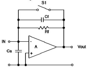
Figure 2-Functional schematic, the charge amplifier
