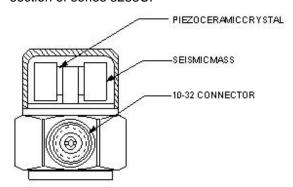
Figure 1-Cross section, series 3255C
