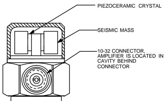
**Figure 1-Cross section, series 3055D**
