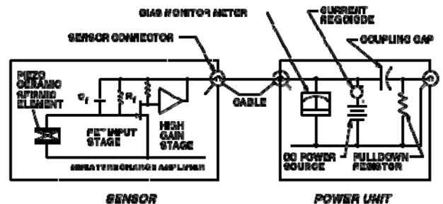
**Figure 2-Electro-mechanical schematic, accelerometer and power unit system.**
