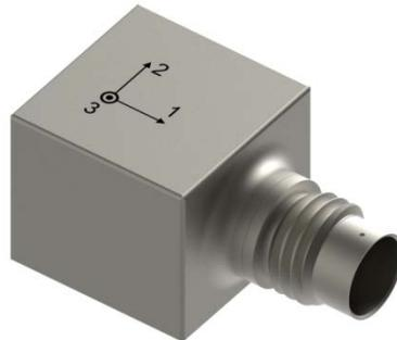
Models 3263AXT are low-noise, miniature IEPE triaxial accelerometers featuring a single, transverse mounted, 4-pin electrical connector. This feature allows the sensor to be used in situations where vertical space is limited. Model series 3263AT is case grounded and available with sensitivities of 10mV/g, 50mV/g, or 100mV/g.
