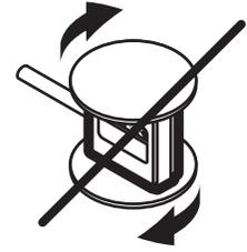
In an environment with a high amount of moisture or humidity, create a drip loop on the cable to prevent any water from flowing into the sensor.
