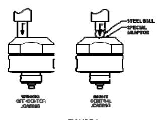
FIGURE 3 ILLUSTRATING OFF-CENTER LOADING
