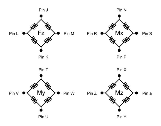
Bridge Fz = 700 ohms Bridges Fx; Fy; Mx; My; Mz = 350 ohms **Connector Type:** Souriau 851-02E16-26P50-44
