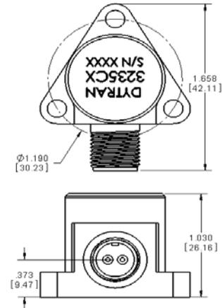
Units on the line drawing are in inches, units in brackets are in millimeters. Refer to 127-3235C for more information.
