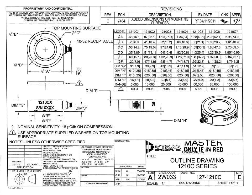
**Model Number** Doc No PERFORMANCE SPECIFICATION PS1210C6 1210C6 Force Sensors, Charge Mode REV C, ECN 11776, 02/27/15
