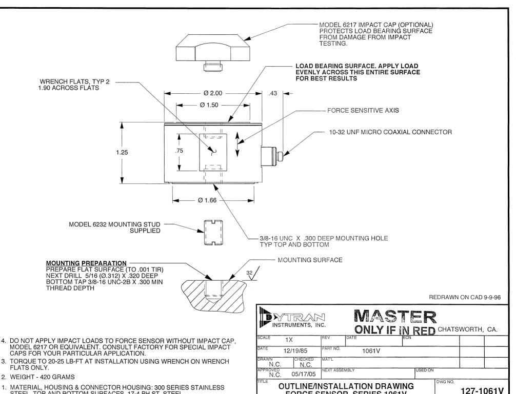
STEEL. TOP AND BOTTOM SURFACES, 17-4 PH ST. STEEL
