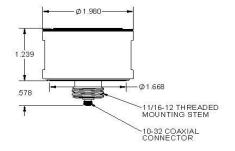
Units on the line drawing are in inches, units in brackets are in millimeters. Refer to 127-1060V for more information.
