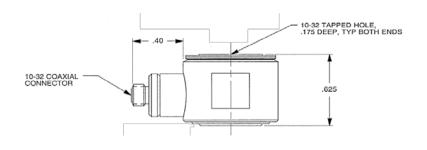
Units on the line drawing are in inches, units in brackets are in millimeters. Refer to 127-1053V for more information.
