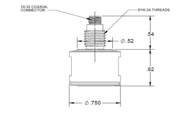
Units on the line drawing are in inches, units in brackets are in millimeters. Refer to 127-1050V for more information.
