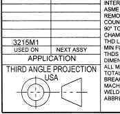
UNLESS OTHERWISE SPECIFIED: INTERPRET DIM & TOL PER ASME Y14.5M - 1994. REMOVE BURRS. COUNTERSINK INTERNAL THDS 90° TO MAJOR DIA. CHAM EXT THDS 45° TO MINOR DIA. THD LENGTHS AND DEPTHS ARE FOR MIN FULL THDS. THDS PER MIL-S-7742 DIMENSIONS APPLY AFTER FINISHING. ALL MACHINED SURFACES. TOTAL RUNOUT WITHIN .005 BREAK SHARP EDGES .005 TO .010. MACHINED FILLET RADII .005 TO .015. WELDING SYMBOLS PER AWS A2.4. ABBREVIATIONS PER MIL-STD-12.
