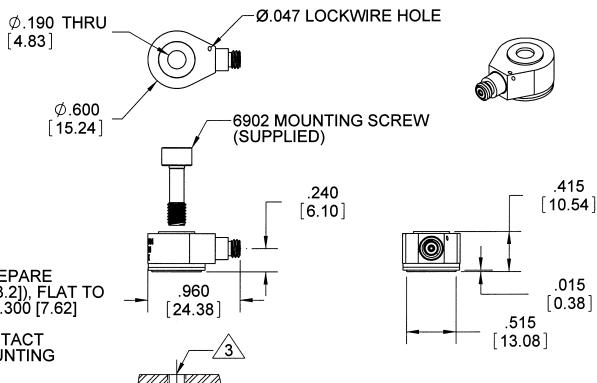
MOUNTING RECOMENDATIONS: PREPARE MOUNTING SURFACE Ø.56 [14.2] (Ø.52 [13.2]), FLAT TO .001 TIR. DRILL AND TAP 10-32 UNC-2B X .300 [7.62] DEEP MIN. RECOMMENDED MOUNTING TORQUE: 15 LB IN +5/-0 LB IN. MUST CONTACT MOUNTING SURFACE OVER ENTIRE MOUNTING SURFACE OF ACCEROMETER.
